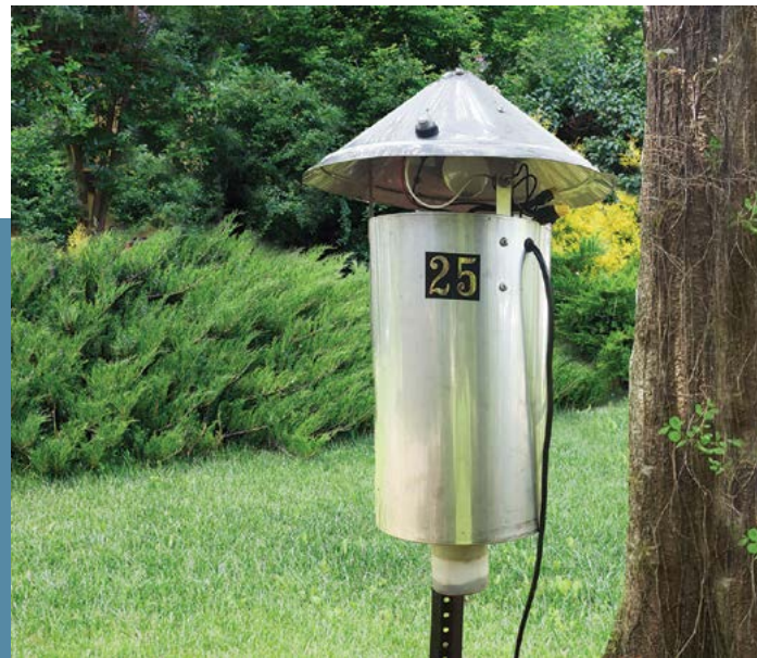
A New Jersey Light Trap is used for mosquito surveillance.
