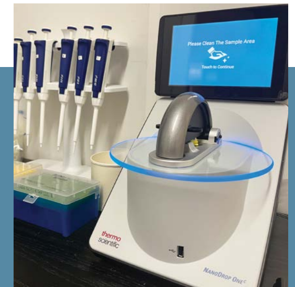
TASD purchased a nanodrop spectrophotometer for determining quality and quantity of nucleic acids and proteins.
