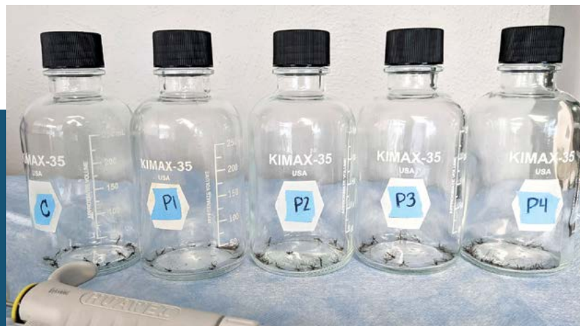
The CDC's bottle bioassay is used for early detection of pesticide resistance in mosquitoes. Glass bottles are coated with pesticides such as permethrin.
