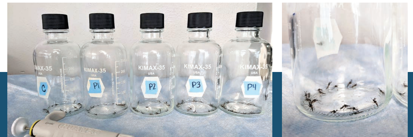
The CDC's bottle bioassay is used for early detection of pesticide resistance in mosquitoes. Glass bottles are coated with pesticides such as permethrin (left). The mortality of approximately 100 mosquitoes is monitored for two hours (right). If more than 4% of the mosquitoes tested survive past the diagnostic time, the population is considered to be potentially resistant.
