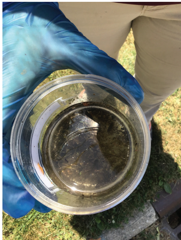
A TASD employee samples catch basin water to determine if granular treatments were effective.
